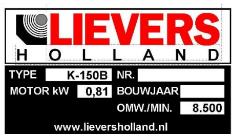
Fig 1: Type plate K-150 The type plate can be found on the motor.
