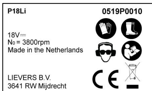
Figure 1: example label P18Li poker vibrator
